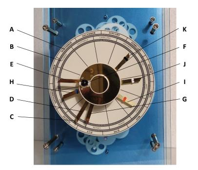
There are two scales on the Dial. The outer scale is calibrated in days; the inner scale is calibrated in degrees.
